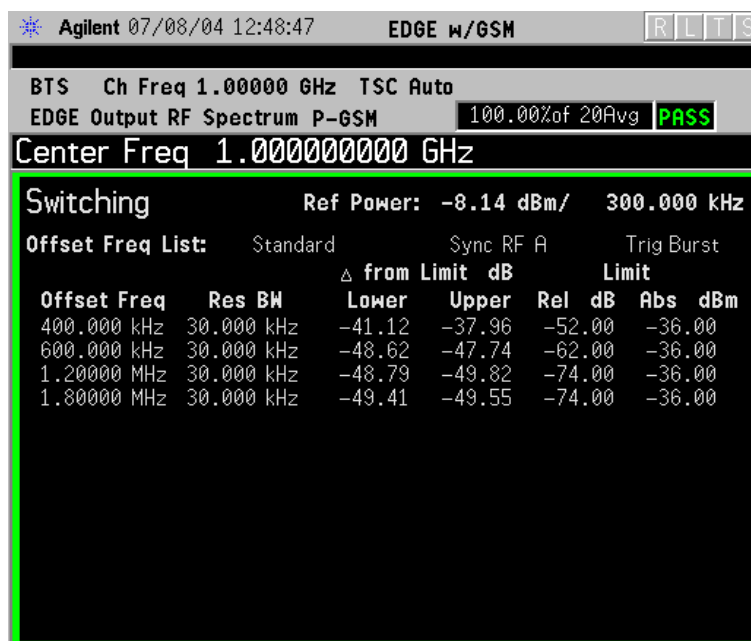
Figure 2-14 EDGE ORFS Result - Switching Margin & Limits View
