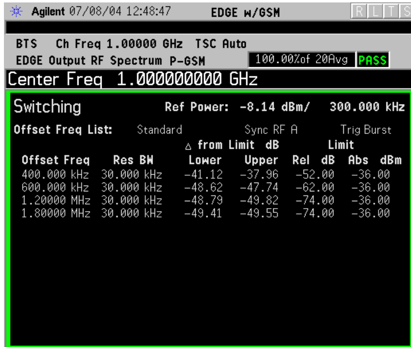
Figure 3-10 EDGE ORFS Result - Example (Short List) Switching Margin & Limits View
