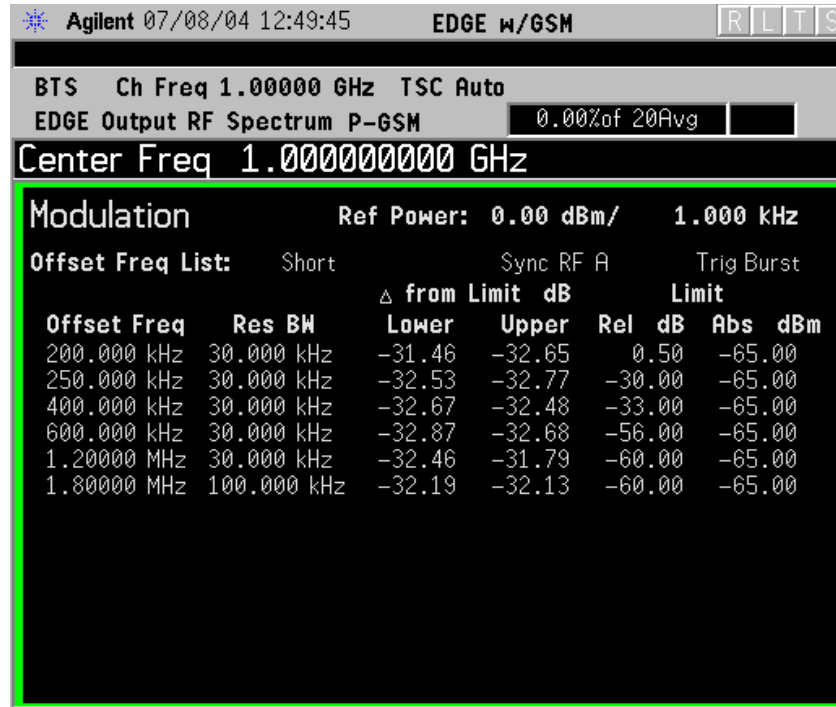
Figure 3-8 EDGE ORFS Result - Example (Short List) Modulation Margin & Limits View
